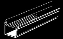
With a **continuous hanger™**, the rain gutters are reinforced along their entire length.
