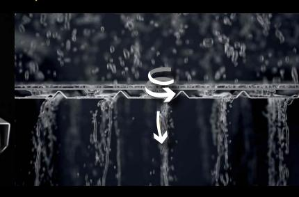
With the **vortex**<sup>TECHNOLOGY</sup>, the suction created by the two membranes makes it possible to drain three times more water than recorded in the heaviest storms.
